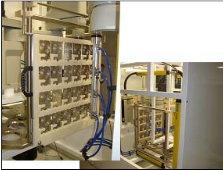
Figure 5. Automated CO 2 composite spray cleaning system.
